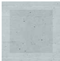
outer: concrete inner: impregnated concrete
