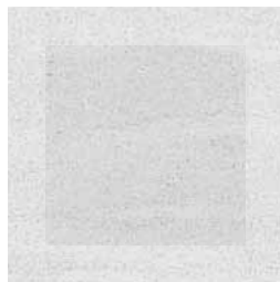
outer: gypsum inner: impregnated gypsum
